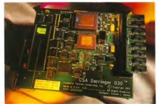
The Derringer fits into the 68000 socket inside the A500, and doesn't take up any of the expansion slots.
